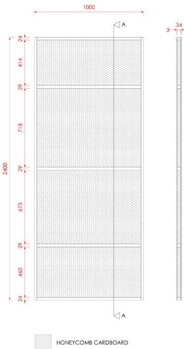
**TIP:** To hold items best, screw directly into the horizontal struts shown in the diagram on the right.
