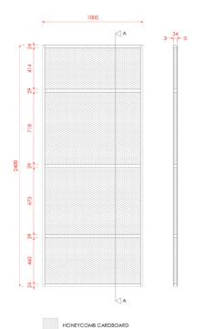
**TIP:** To hold items best, screw directly into the horizontal struts shown in the diagram on the right.
